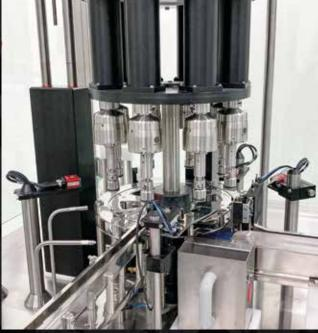
FD120SA model is an alternate motion Machine for test tubes production to be used for preparation swab nasopharyngeal tests and testing Viruses (Ex. COVID 19).
