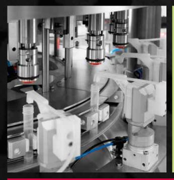
RFC16SA model is a continuous motion test tubes line to be used for preparation swab nasopharyngeal tests and testing Viruses (Ex. COVID-19).
