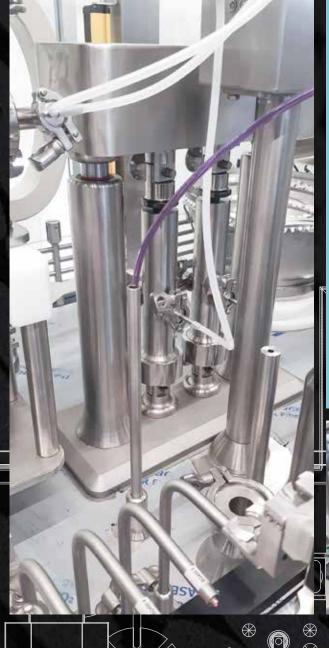
The new RSL model is a versatile, double index machine, designed to fill and close most pharmaceutical containers especially ophthalmic and injectables.
